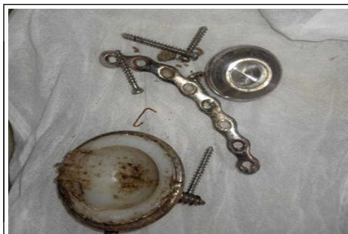
Figure 3: Recovered prosthesis with damaged ball.
