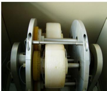
Figure 1: The main HSCCC multi-layer coil separation columns.
