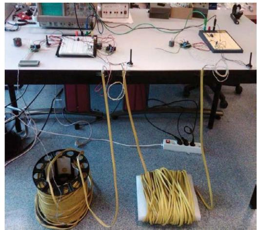
Figure 6: The Transmitter and Receiver Coupled to the DC bus.
