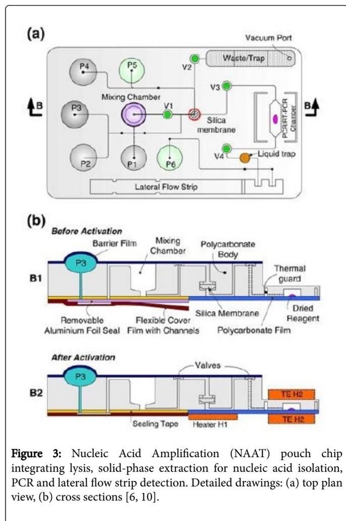
**Figure 3:** Nucleic Acid Amplification (NAAT) pouch chip integrating lysis, solid-phase extraction for nucleic acid isolation, PCR and lateral flow strip detection. Detailed drawings: (a) top plan view, (b) cross sections [6, 10].
