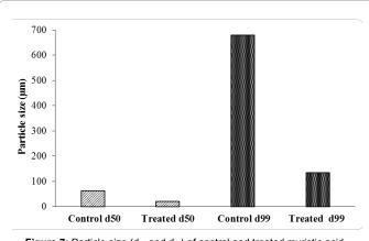
Figure 7: Particle size (d<sub>50</sub> and d<sub>99</sub>) of control and treated myristic acid.
