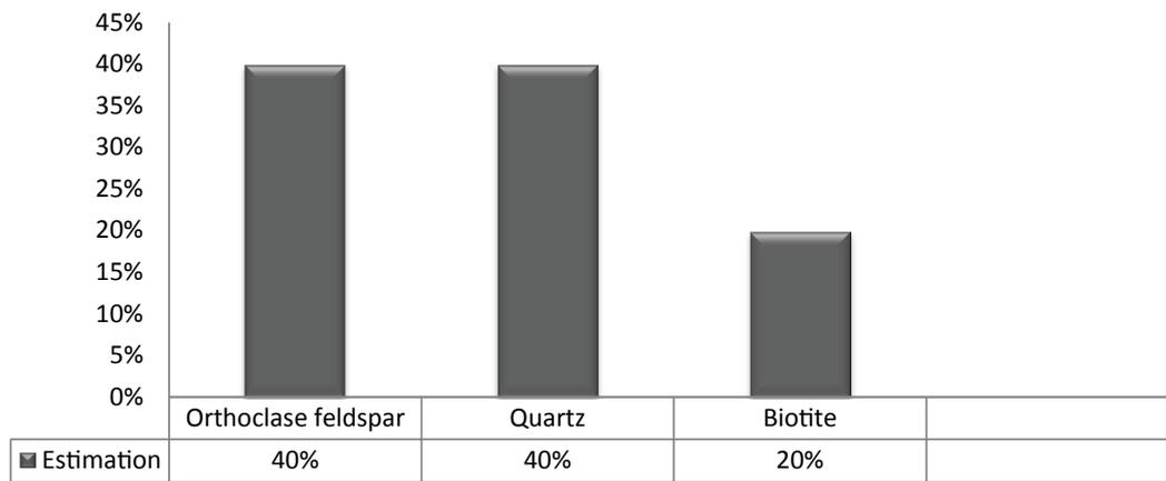
Figure 7: Bar chart showing estimated modal mineralogical composition of granite under the microscope.
