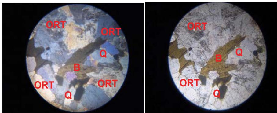
Figure 6: Photomicrograph of granite showing its mineralogical composition in XPL and PPL (B =Biotite, Q=Quartz and ORT=Orthoclase) (a) SM1 PP M40 (b) SM1 XP M40.
