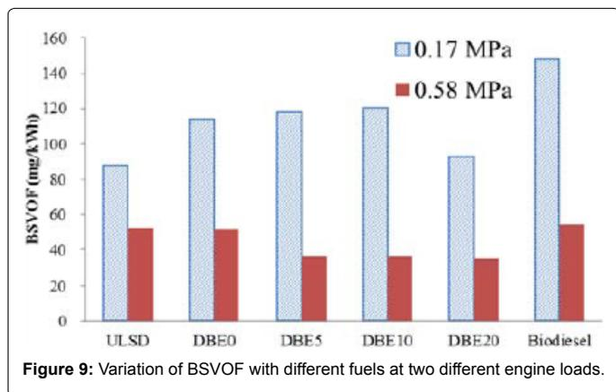
Figure 9: Variation of BSVOF with different fuels at two different engine loads.
