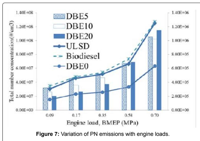
is generally observed to achieve the highest PN because of its higher fuel viscosity favoring higher production of smaller particles. The DBE blends with ethanol could reduce PN by 99% on average for all engine loads as compared with both biodiesel and ULSD. It is due to the combined effect of the oxygen content and the alcohol structure in ethanol which is effective in reducing soot precursors.
