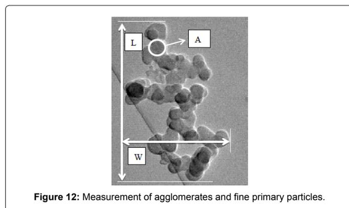
Figure 12: Measurement of agglomerates and fine primary particles.
