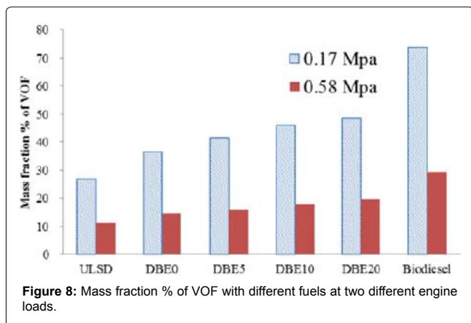
Figure 8: Mass fraction % of VOF with different fuels at two different engine loads.
