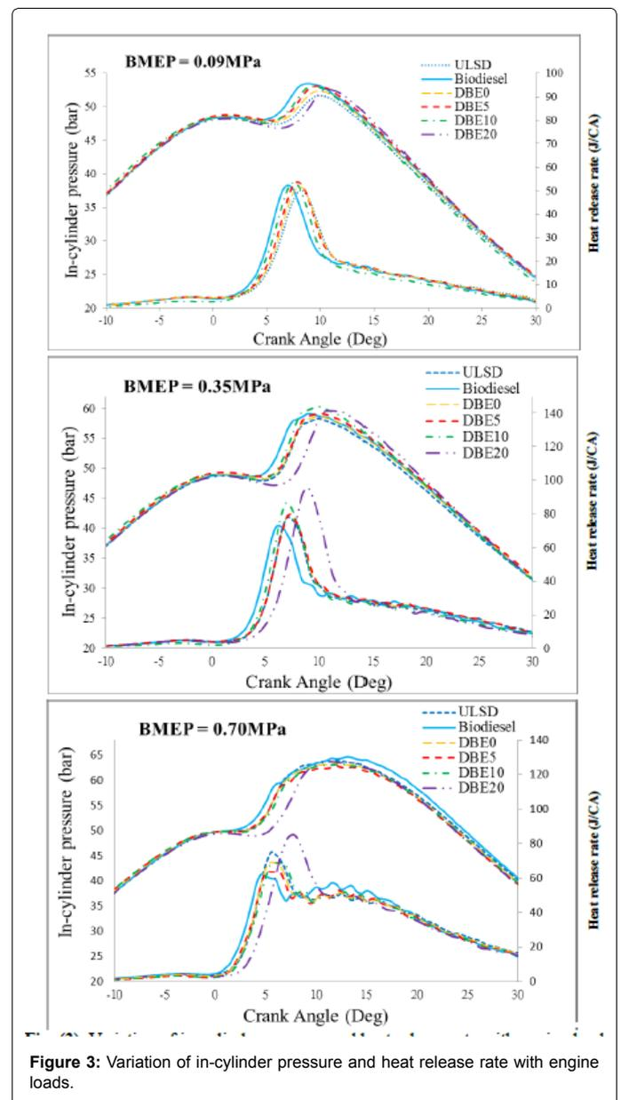
Figure 3: Variation of in-cylinder pressure and heat release rate with engine loads.
