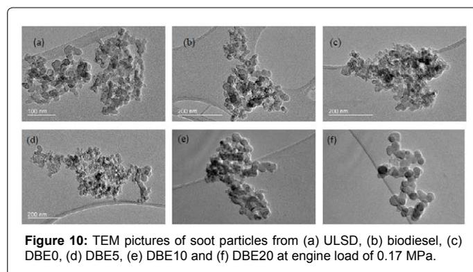
Figure 10: TEM pictures of soot particles from (a) ULSD, (b) biodiesel, (c) DBE0, (d) DBE5, (e) DBE10 and (f) DBE20 at engine load of 0.17 MPa.
