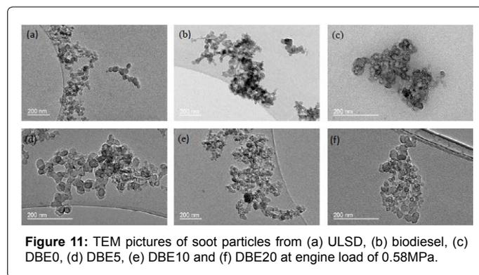
Figure 11: TEM pictures of soot particles from (a) ULSD, (b) biodiesel, (c) DBE0, (d) DBE5, (e) DBE10 and (f) DBE20 at engine load of 0.58 MPa.
