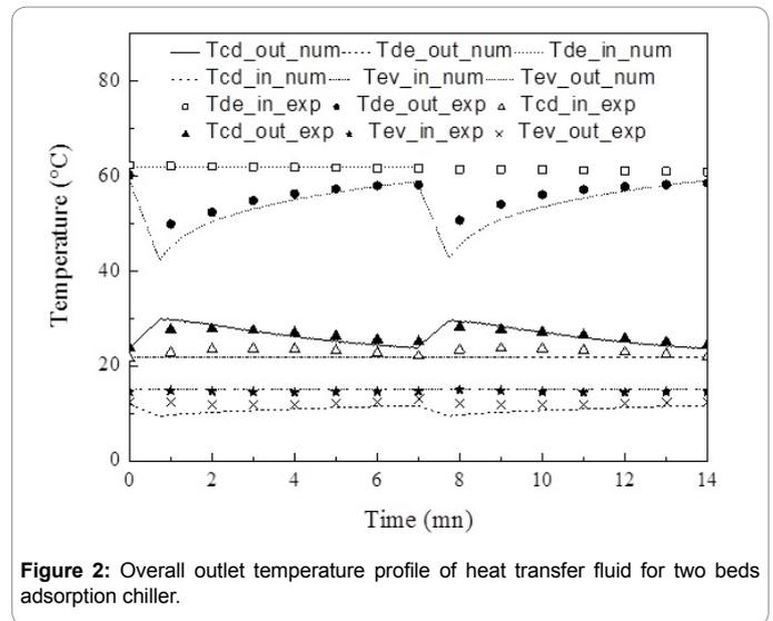
Figure 2: Overall outlet temperature profile of heat transfer fluid for two beds adsorption chiller.
