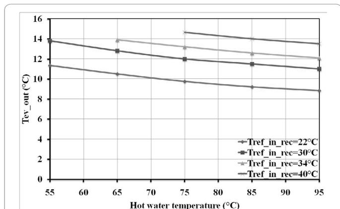
Figure 4: Generation temperature influence on  $T_{ev\_out}$  ( $T_{ev\_in}=15^{\circ}\text{C}$ ,  $t_{cycle}=840$  s).
