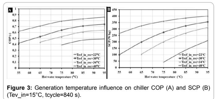
Figure 3: Generation temperature influence on chiller COP (A) and SCP (B) ( $T_{ev,in}=15^\circ\text{C}$ ,  $t_{cycle}=840$  s).
