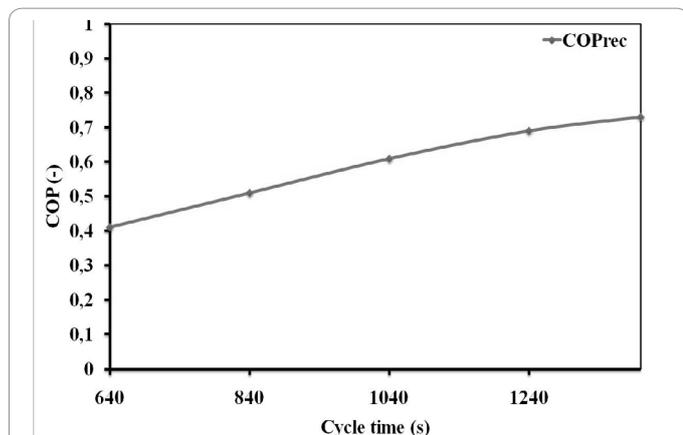
Figure 8: Effect of cycle time on the COP ( $T_{de\_in}=85^{\circ}\text{C}$ ,  $T_{ref\_in}=40^{\circ}\text{C}$ ,  $T_{ev\_in}=15^{\circ}\text{C}$ ).
