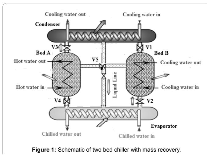
Figure 1: Schematic of two bed chiller with mass recovery.
