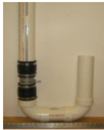
Figure 2: Constructed a device for a hydraulic conductivity test.
