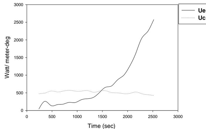
Figure 5 Variation in overall heat transfer coefficients, “ $U_c$ ” over condenser and “ $U_e$ ” over evaporator
