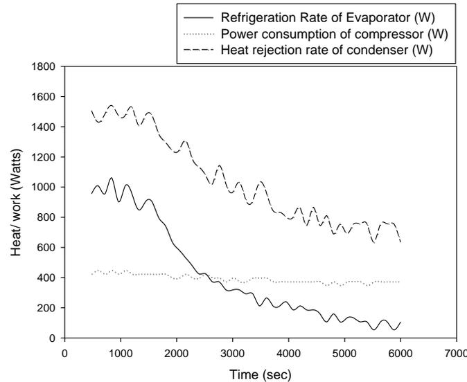
Figure 4 : Performance of VCR system under transient conditions
