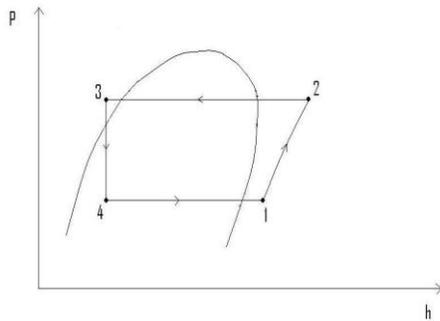
Figure 2 : Theoretical vapour compression cycle
