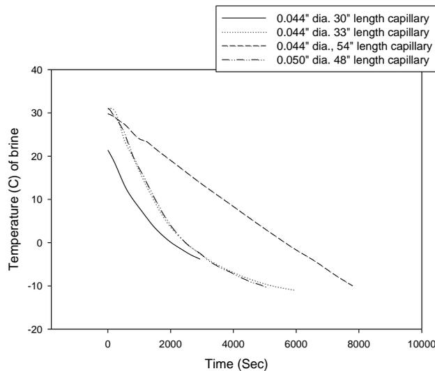
Figure 7 Fall of temperature of brine in evaporator shell with time
