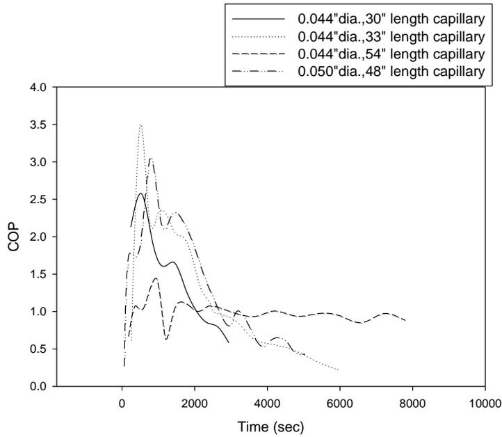
Figure 6 Variation in actual COP with different sizes of capillary tube under transient conditions
