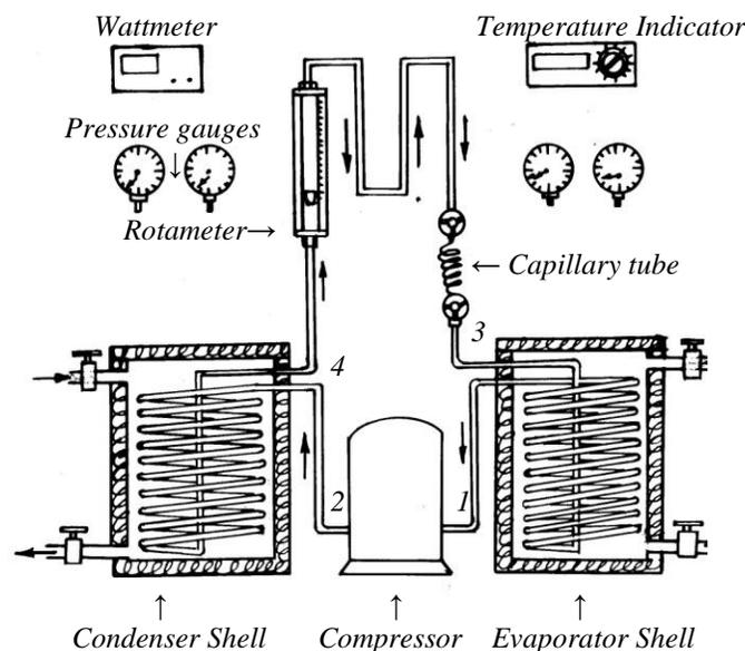
Figure 1 Experimental set up of simple vapour compression refrigeration system
