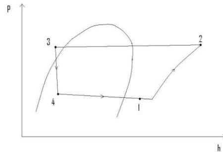
Figure 3: Actual vapour compression cycle
