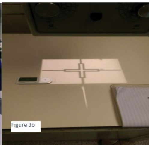
Figure 3: (a) Image showing setup of R/F detector at a projected field height. (b) Image showing setup of the portable R/F detector at tabletop.
