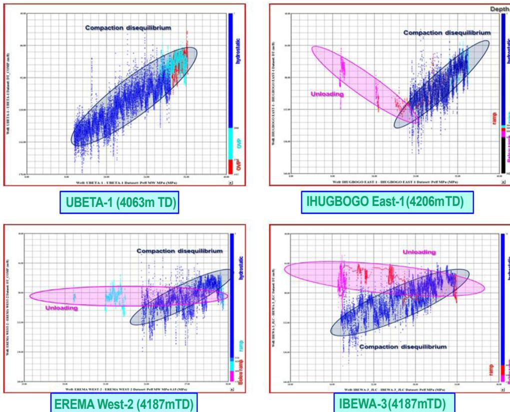
Figure 1a: Sonic (DT) versus Pseudo-Effective Stress (OBG-MW) cross-plots.
