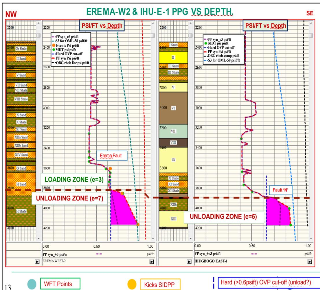
Figure 1b: Pressure versus depth plots of deep objective targeting wells in Block "X". Note the need change the Eaton's co-efficient in the hard overpressure zone.
