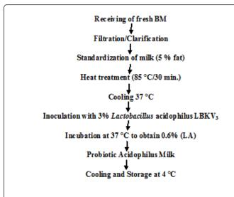
**Figure 1:** Flow diagram for manufacture of Probiotic Acidophilus Milk.
