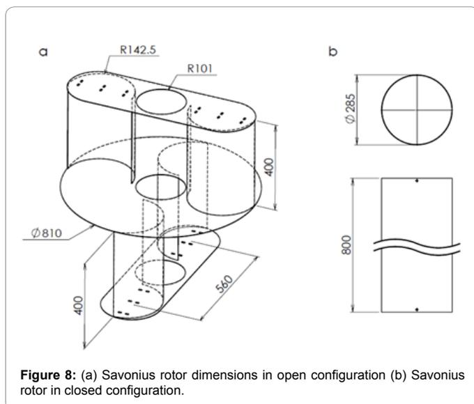
Figure 8: (a) Savonius rotor dimensions in open configuration (b) Savonius rotor in closed configuration.
