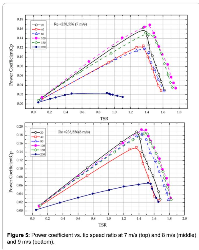
Figure 5: Power coefficient vs. tip speed ratio at 7 m/s (top) and 8 m/s (middle) and 9 m/s (bottom).
