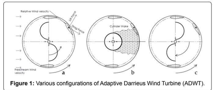
Figure 1: Various configurations of Adaptive Darrieus Wind Turbine (ADWT).
