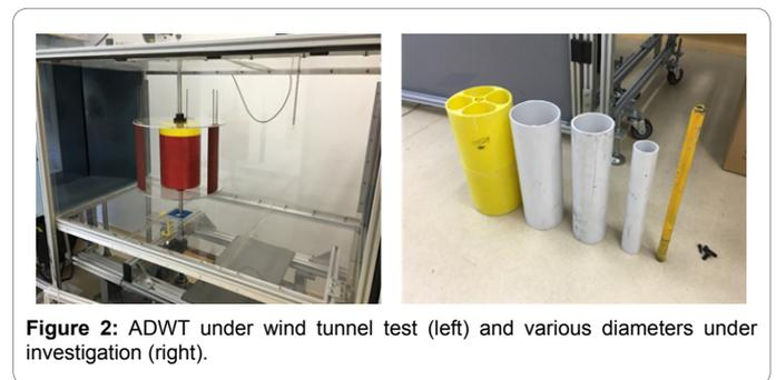
Figure 2: ADWT under wind tunnel test (left) and various diameters under investigation (right).
