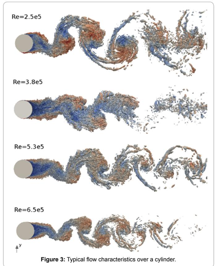
Figure 3: Typical flow characteristics over a cylinder.
