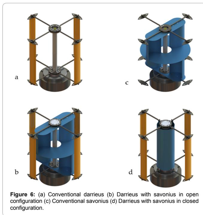
Figure 6: (a) Conventional darrieus (b) Darrieus with savonius in open configuration (c) Conventional savonius (d) Darrieus with savonius in closed configuration.
