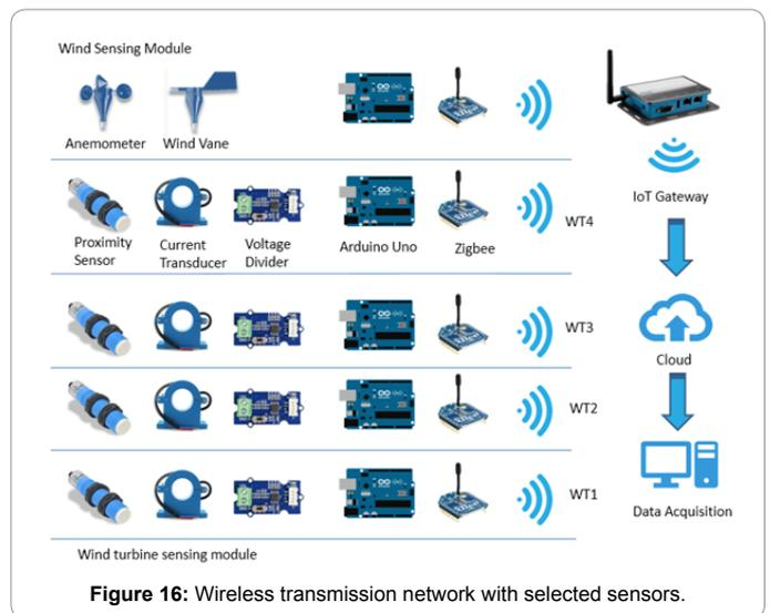
Figure 16: Wireless transmission network with selected sensors.
