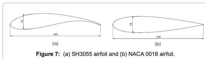
Figure 7: (a) SH3055 airfoil and (b) NACA 0018 airfoil.
