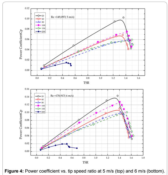
Figure 4: Power coefficient vs. tip speed ratio at 5 m/s (top) and 6 m/s (bottom).
