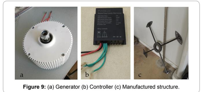
Figure 9: (a) Generator (b) Controller (c) Manufactured structure.
