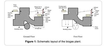
gas tight. The sewage from the toilets was piped to the influent port of the biogas plant while wastewater from the baths/shower (where a lot of soaps and detergents are used) was piped directly into the septic tank without passing through the biogas reactor. The effluent from the reactor was discharged into the already existing septic tank/soak away.
