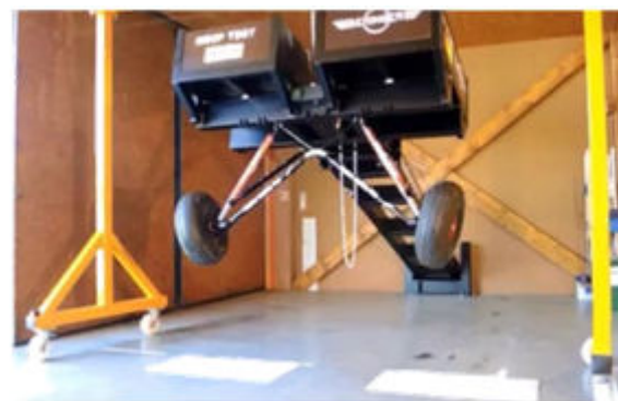
Figure 11: Drop test session on light aircraft landing gear [11].
