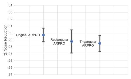
Figure 6: Percent noise reduction of three ARPRO geometries for the high-frequency tests, N=30.
