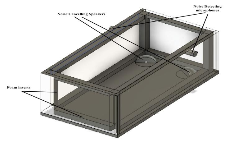
Figure 1: 3D Model of foam inserts with noise-canceling speakers.
