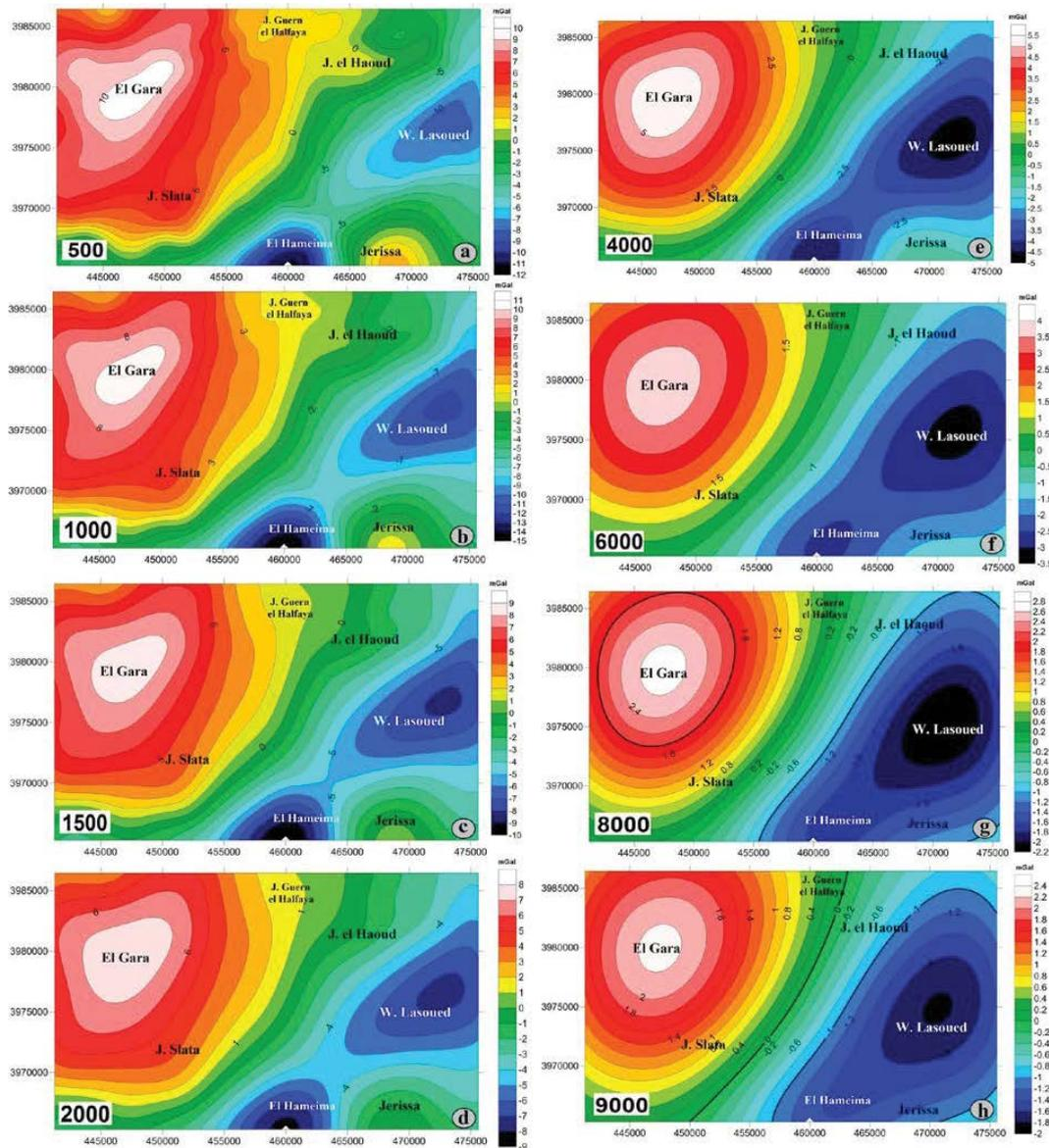
**Figure 6 a-h:** Upward continuation of the Bouguer anomaly maps at several heights: 500 m (a); 1000 m (b); 1500 m (c); 2000 m (d); 4000 m (e); 6000 m (f); 8000 m (g) and 9000 m (h).
