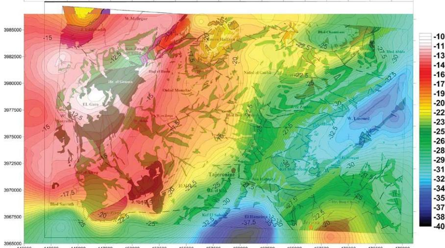
Figure 5: Superposed Bouguer anomalies map on the geological map.
