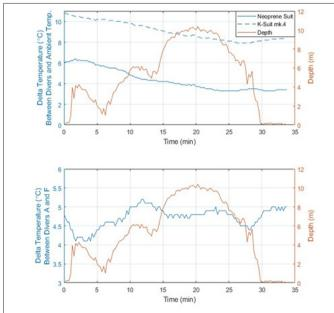
**Figure 2:** Dive Test #1. Diver A wearing the K<sub>2</sub> prototype and Diver F wearing a 5 mm commercial neoprene suit performed a tandem dive, with the above results. **Note:** (–) Neoprene Suit, (––) K2 suit, (–) Depth.
