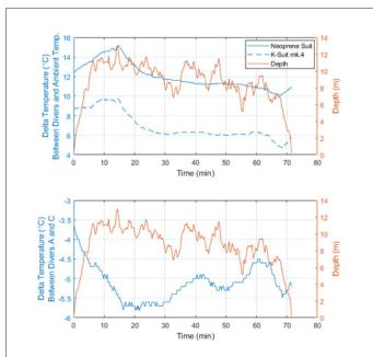
**Figure 4:** Dive Test #3. Diver A wearing the K2 prototype and Diver C wearing a 7 mm neoprene suit and a 3 mm sleeveless neoprene vest performed a tandem dive, with the above results. **Note:** (–) Neoprene Suit, (––) K2 suit, (–) Depth.
