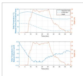
**Figure 5:** Dive Test #4. Diver A wearing the K2 prototype and Diver E wearing a 7 mm neoprene Long-John suit and a 7 mm neoprene jacket suit performed a tandem dive, with the above results. **Note:** (–) Neoprene Suit, (––) K2 suit, (–) Depth.
