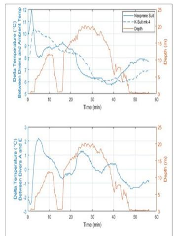
**Figure 3:** Dive Test #2. Diver A wearing the K<sub>2</sub> prototype and Diver E wearing a 7mm commercial neoprene suit performed a tandem dive, with the above results. **Note:** (–) Neoprene Suit, (––) K2 suit, (–) Depth.
