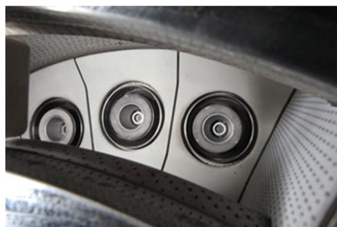
Figure 4: GE N+2 5-cup CMC combustor sector rig.
