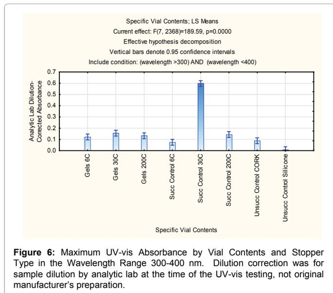
Figure 6: Maximum UV-vis Absorbance by Vial Contents and Stopper Type in the Wavelength Range 300-400 nm. Dilution correction was for sample dilution by analytic lab at the time of the UV-vis testing, not original manufacturer's preparation.
