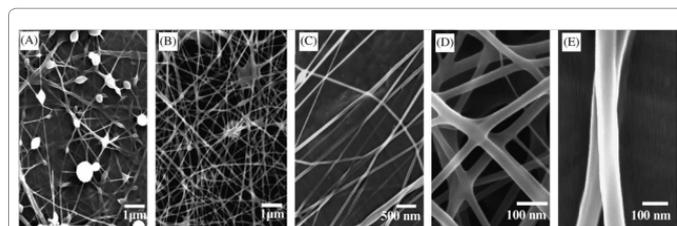
**Figure 5:** SEM images of electrospun structures (chitosan/PEO ratio 90/10) prepared from aqueous solution containing 0.5M acetic acid: (A) 0.3% Triton X-100™, (B) and (C) 0.3% Triton X-100™ and 10% DMSO. Fibers in (B) were collected on a stationary collector whereas fibers in (C) were collected on a cylindrical collector with a rotating speed of 2000 rpm. Images (D) and (E) are the high-magnification images of (B) and (C), respectively. (from ref [49] with permission).
