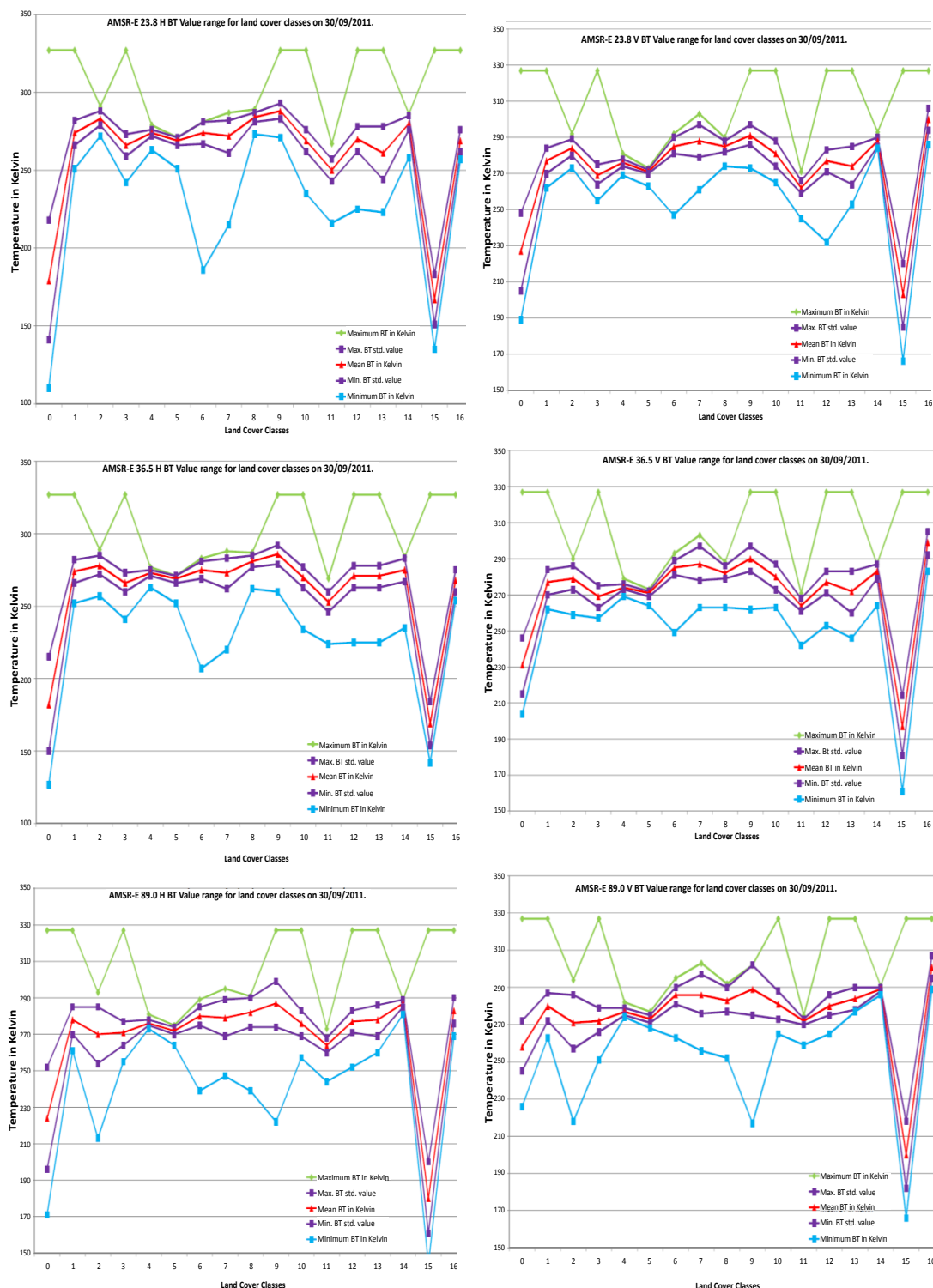
Figure 2: Seventeen land cover classes maximum, minimum, mean and standard deviation temperature in kelvin for 6.9, 10.7, 18.7, 23.8, 36.5 and 89.0 Ghz AMSR-E frequency.
