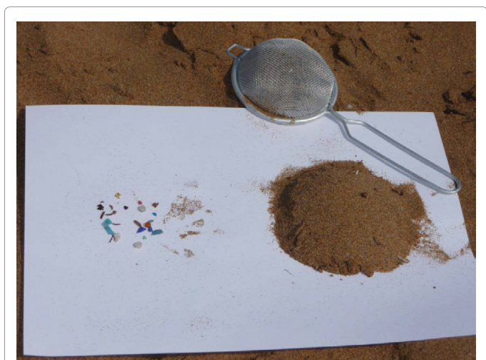
Figure 7: Illustration of the amount of visible microplastics found in beach sand. Photo Vethaak AD.
