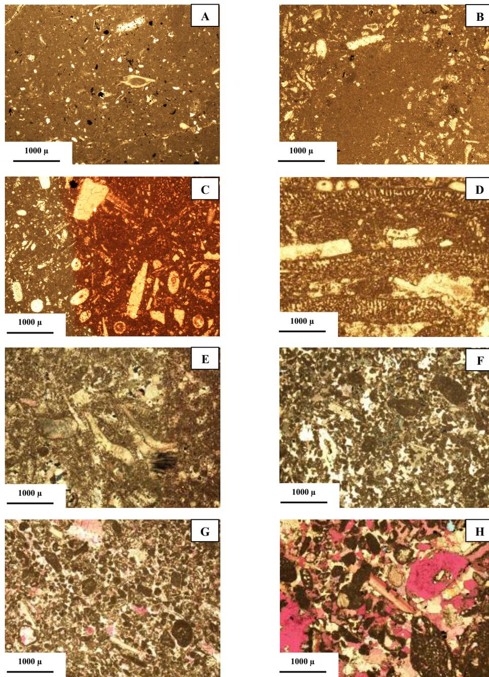
**Figure 2:** Photomicrograph of different microfacies. A: MF1- skeletal wackestone. PPL. B: MF1- skeletal wackestone with bioturbation. PPL. C: MF2- skeletal wackestone to packstone (thin section stained with alizarin red-s). XPL. D: MF3- dolo skeletal packstone. XPL. E: MF4- skeletal packstone with rudist debris. XPL. F: MF4- skeletal packstone to grainstone. G and H: MF5-skeletal grainstone. XPL.
