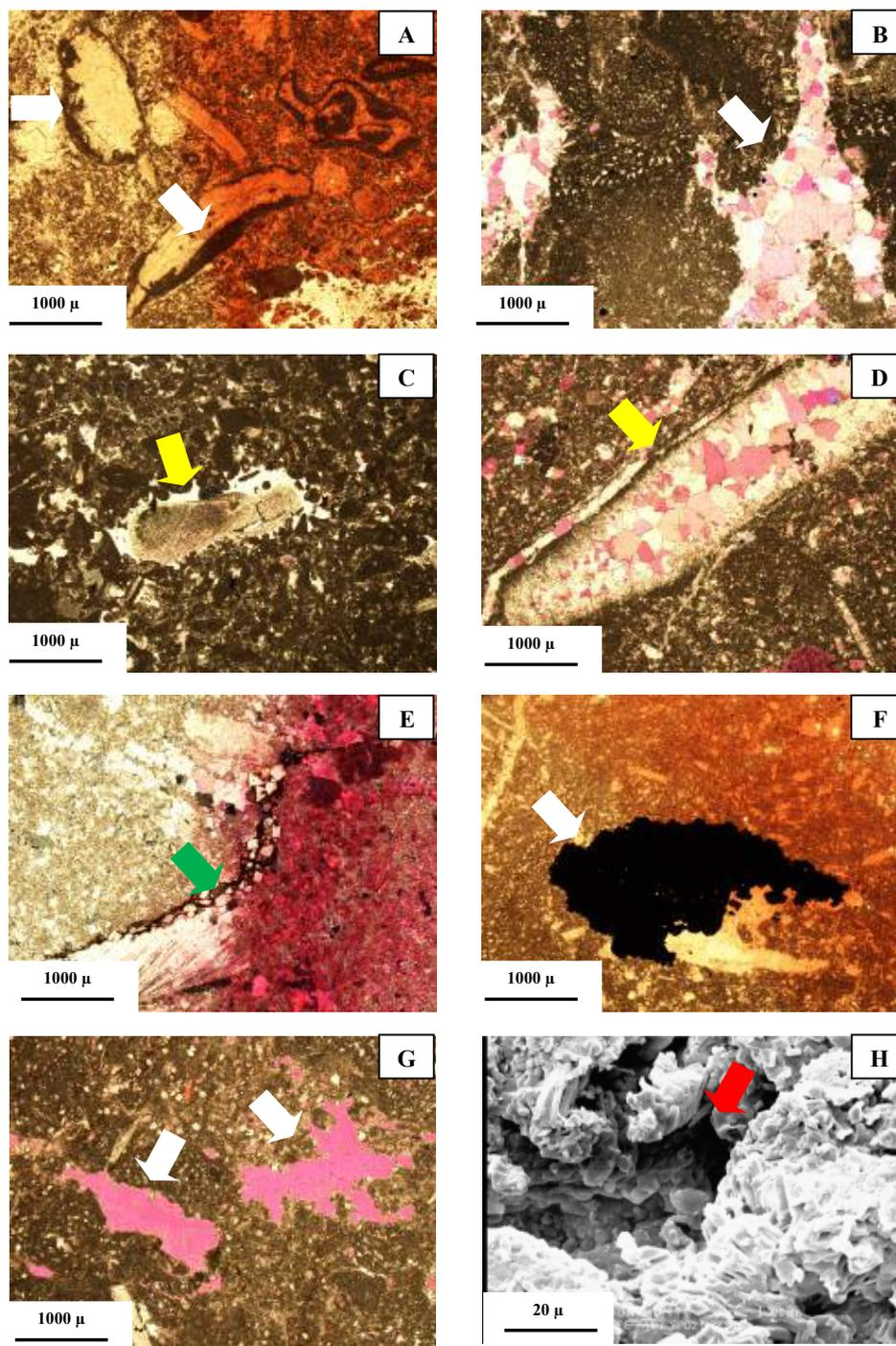
**Figure 4:** Photomicrograph of different diagenetic processes. A: micrite envelope around rudist debris. PPL. B: sparry calcite cement. XPL. C: syntaxial cement around echinoderm debris xpl. D: neomorphism in a skeletal debris, XPL. E: solution seams with crystals of dolomite around it. XPL. F: partial fabric selective pyritization in a shell fragment.ppl. G: vuggy porosity (in purple). XPL. H: SEM photo of microporosity.
