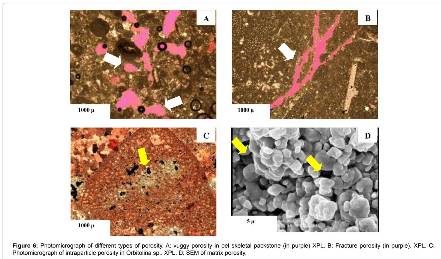
**Figure 6:** Photomicrograph of different types of porosity. A: vuggy porosity in pel skeletal packstone (in purple) XPL. B: Fracture porosity (in purple). XPL. C: Photomicrograph of intraparticle porosity in *Orbitolina* sp.. XPL. D: SEM of matrix porosity.
