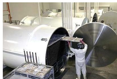
Figure 15: Industrial freeze dryer [125].
