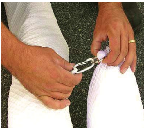
Figure 3: Metal clips link sorbent booms together for extra length.
