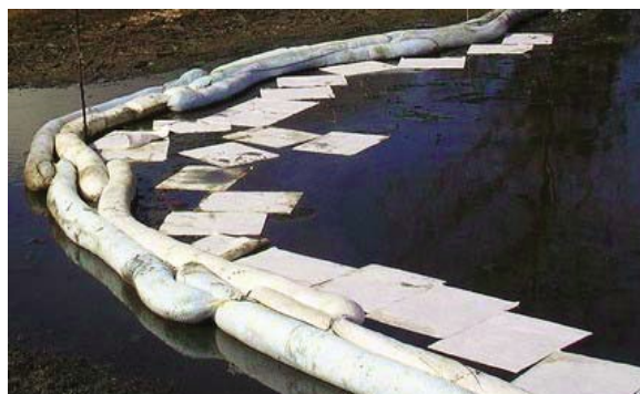
Figure 7: Spread the sorbent pads on the surface to collect the spillage.
