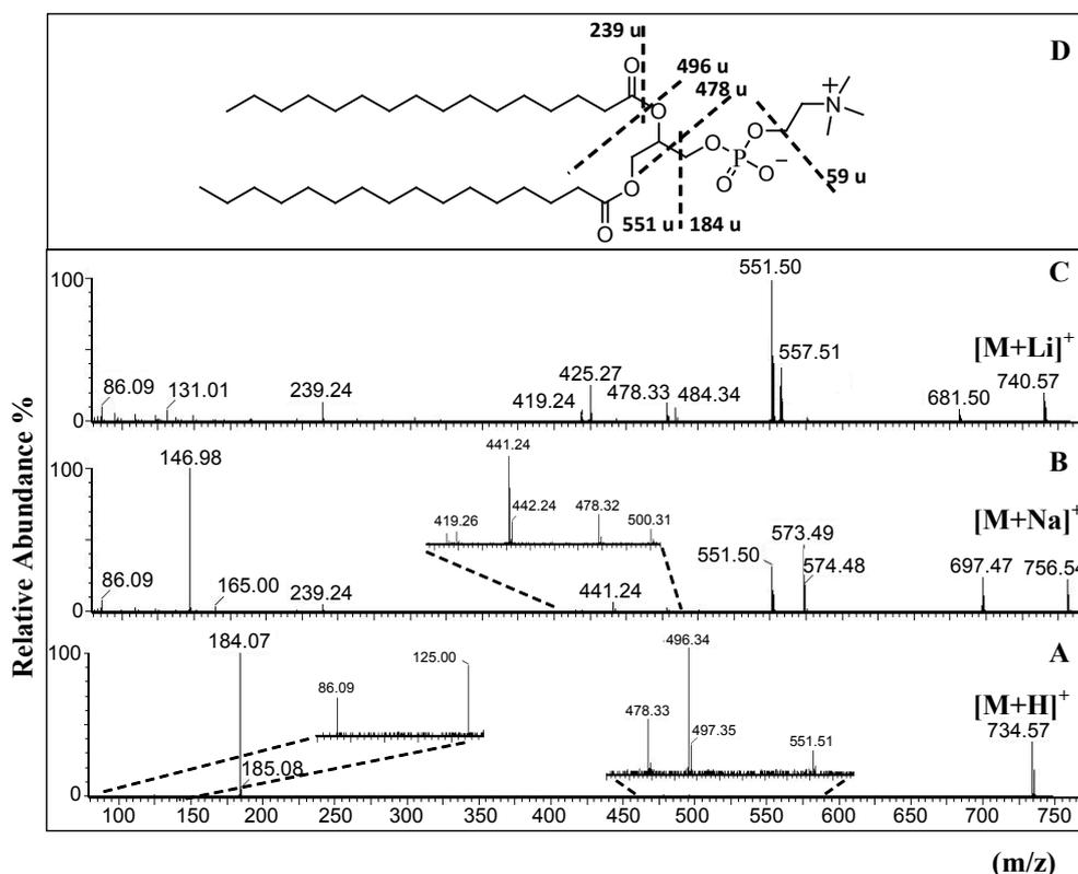
**Figure 1:** MALDI-Q-TOF spectra of DPPC (16:0/16:0) obtained inducing the fragmentation of (a)  $[M+H]^+$  (m/z 734.57), (b)  $[M+Na]^+$  (m/z 756.54), and (c)  $[M+Li]^+$  (m/z 740.57), (d) Scheme of the important fragments observed in figure 1A.
