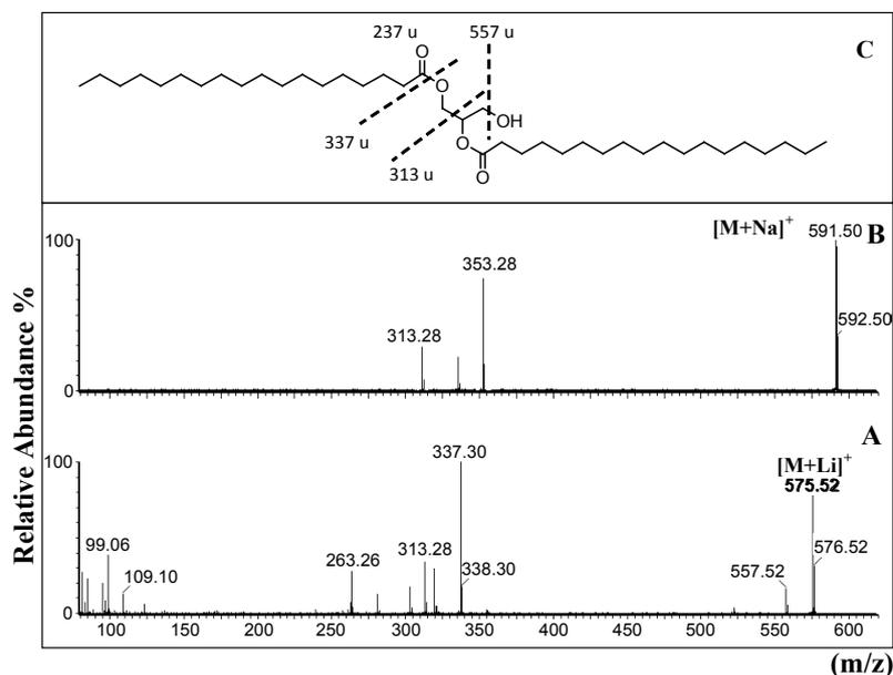
**Figure 7:** MALDI-Q-TOF spectra of PP (16:0/16:0) obtained inducing the fragmentation of (a)  $[M+Li]^+$  ( $m/z$  575.52), (b)  $[M+Na]^+$  ( $m/z$  591.50) and (c) Scheme of the important fragments observed in figure 7A.
