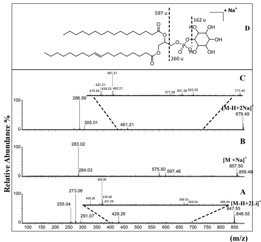
Figure 4: MALDI-Q-TOF spectra of PI obtained inducing the fragmentation of (a)  $[M+2Li-H]^+$  (m/z 847.55), (b)  $[M+Na]^+$  (m/z 857.50), (c)  $[M+2Na-H]^+$  (m/z 879.49) and (d) Scheme of the important fragments observed in figure 4B.
