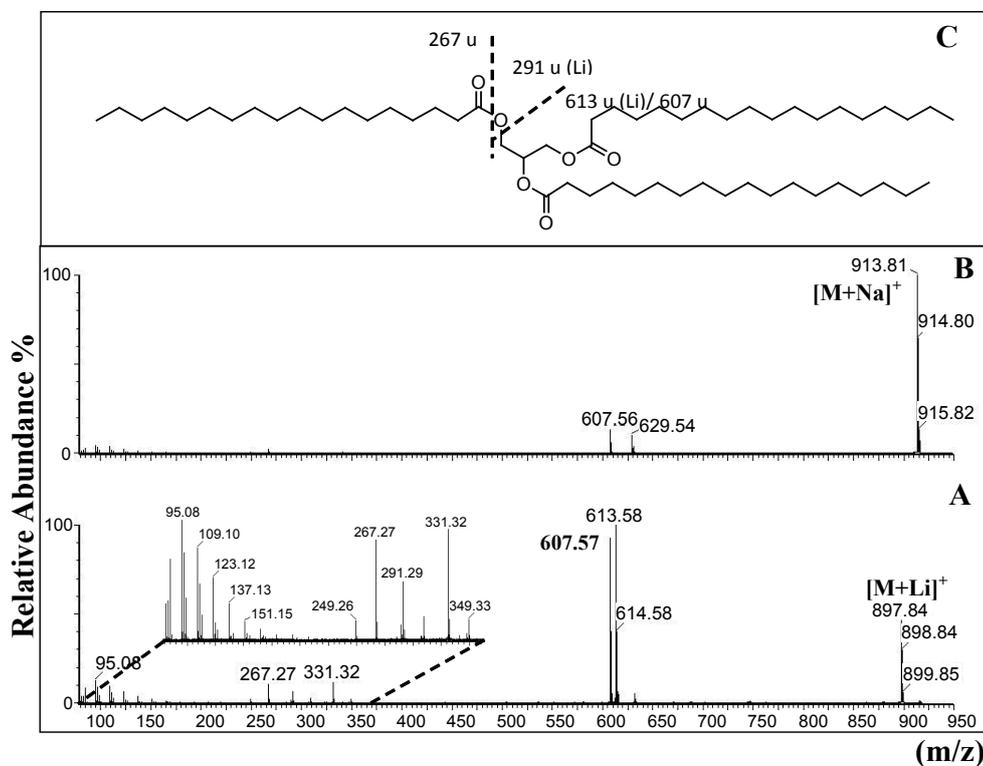
**Figure 6:** MALDI-Q-TOF spectra of SSS (18:0/18:0/18:0) obtained inducing the fragmentation of (a)  $[M+Li]^+$  ( $m/z$  897.84), (b)  $[M+Na]^+$  ( $m/z$  913.81) and (c) Scheme of the important fragments observed in figure 6A.
