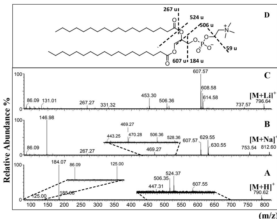
**Figure 2:** MALDI-Q-TOF spectra of DSPC (18:0/18:0) obtained inducing the fragmentation of (a)  $[M+H]^+$  ( $m/z$  790.62), (b)  $[M+Na]^+$  ( $m/z$  812.60), (c)  $[M+Li]^+$  ( $m/z$  796.64), (d) Scheme of the important fragments observed in figure 2A.
