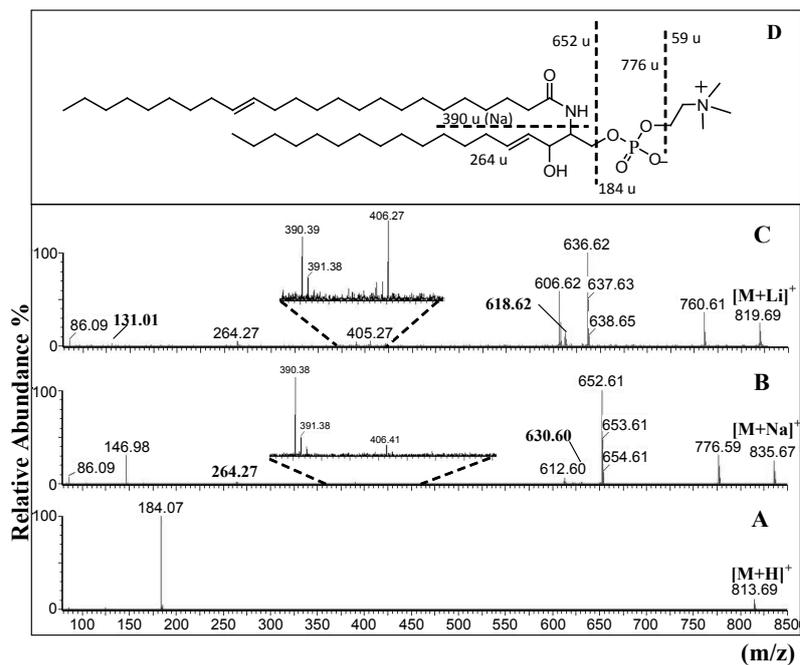
**Figure 5:** MALDI-Q-TOF spectra of SM (18:1/24:1) obtained inducing the fragmentation of (a)  $[M+H]^+$  ( $m/z$  813.69), (b)  $[M+Na]^+$  ( $m/z$  835.67) and (c)  $[M+Li]^+$  ( $m/z$  819.69) and (d) Scheme of the important fragments observed in figure 5B.
