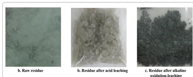
Figure 7: Image of A) Raw residue; B) Residue after acid leaching; C) Residue after alkaline oxidation-leaching.
