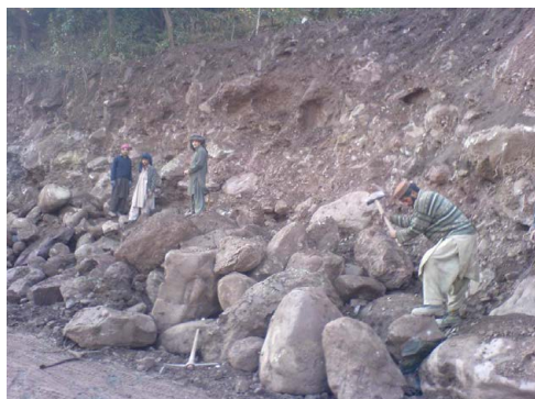
Figure 8: Boulders of volume up to about 0.8-1.2 m 3 has moved down the slopes with debris. The presence of people provides an implication of the relative size.
