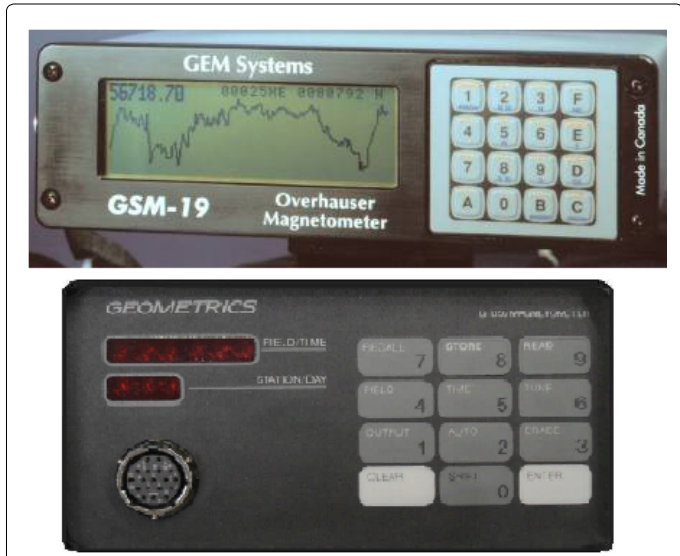
Figure 4: Proton-Precession Magnetometer (G856-AX, [16]) and Overhauser Magnetometer [17].
