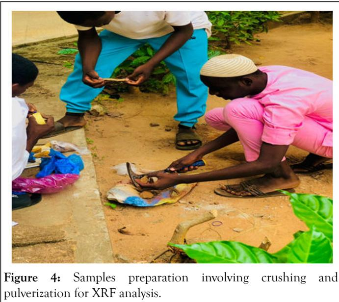
Figure 4: Samples preparation involving crushing and pulverization for XRF analysis.
