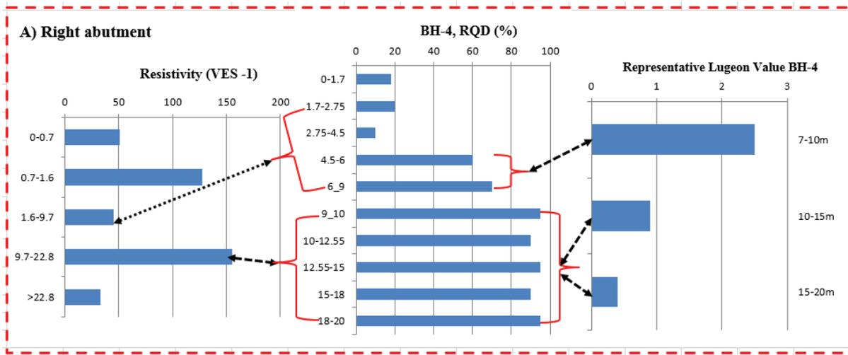
Figure 14: The integrated result of VES, RQD and permeability at the right abutment of the proposed dam.
