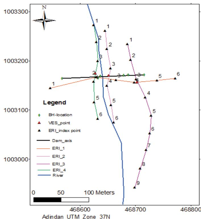
Figure 2: The above figure shows the investigation line on the proposed dam site.
