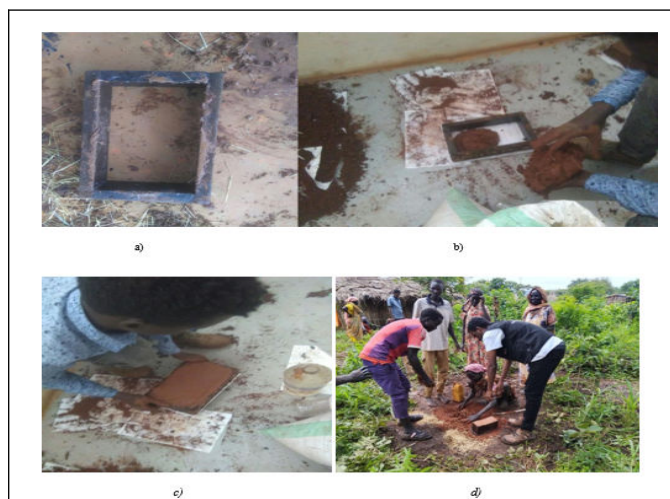
Figure 6: a) Mold to cast the mud; b) Casting the mud using the mold; c) Removing the mold; d) Exposing the mud brick to sunlight.
