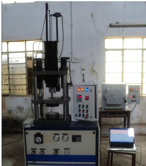
Fig 2: Hydraulic press with die set
