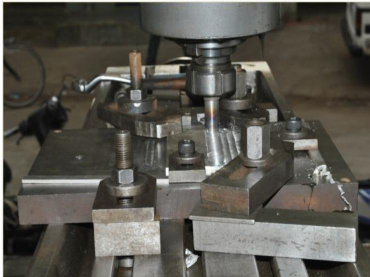
Fig1: Friction stir processing set up
