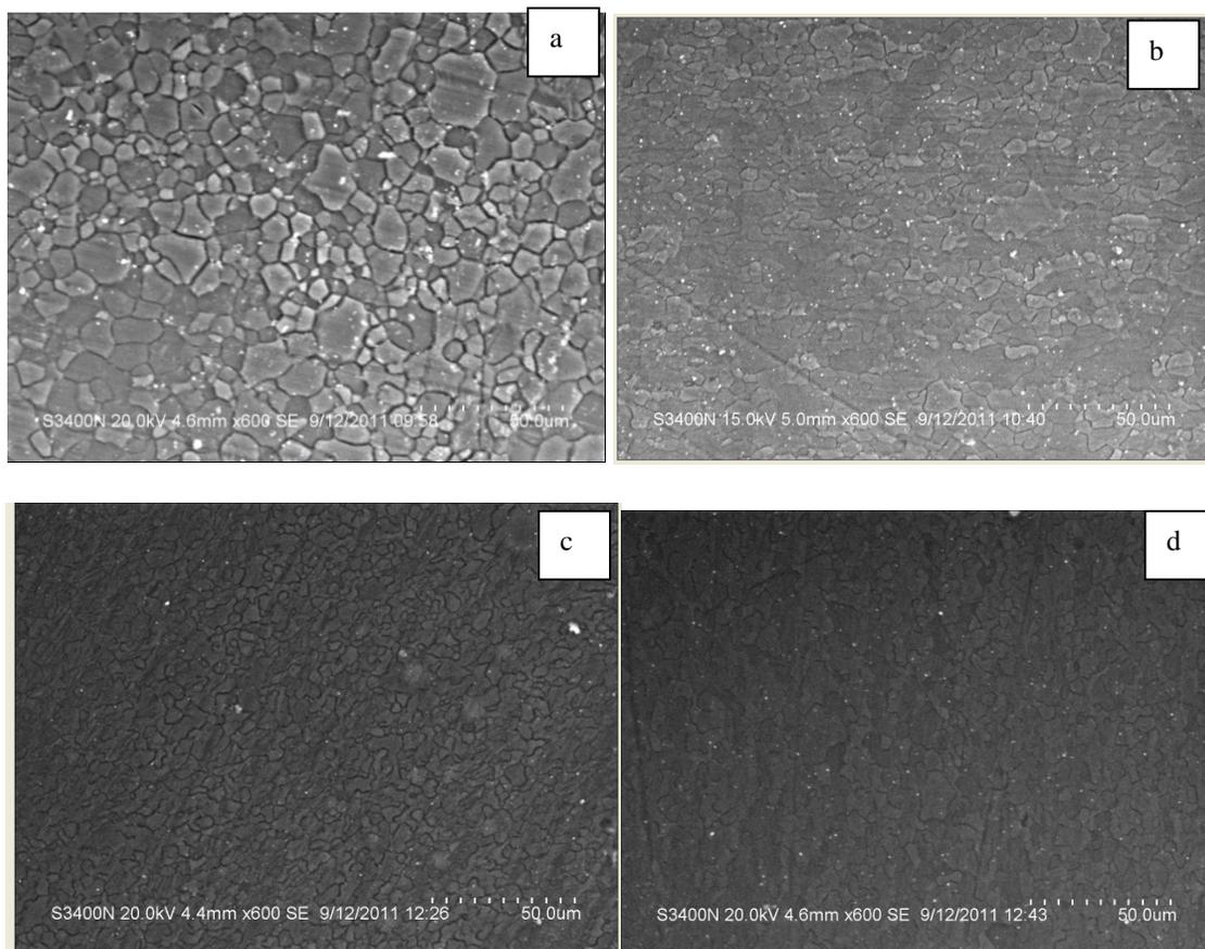
Fig 3: (a) Optical microstructure base material (b) FSPed material at traverse speed of 24mm/min (c) 32mm/min (d) 40mm/min
