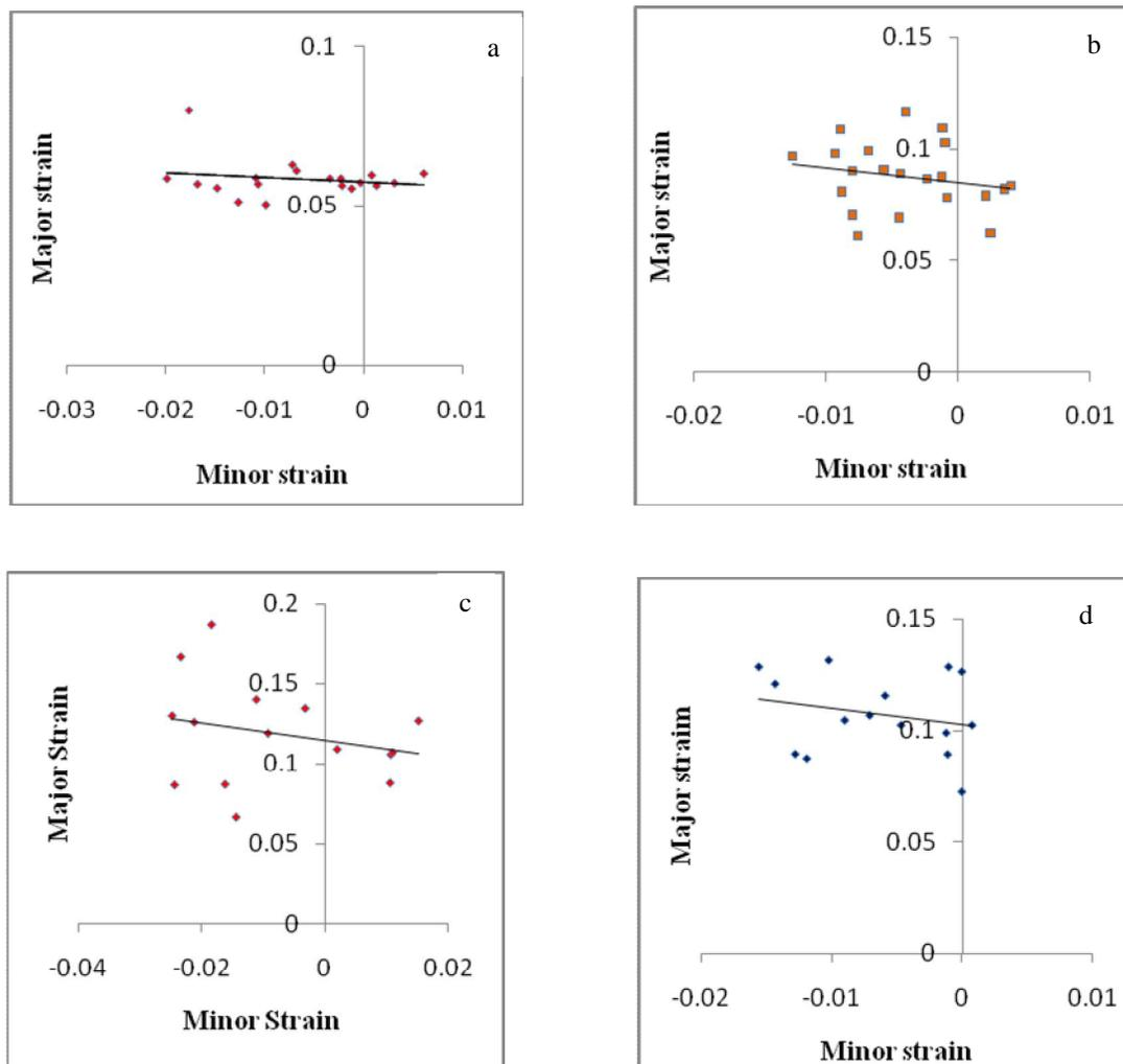
Fig 4: Fracture Limits of (a) base material (b) at T.S of 24mm/min (c) 32mm/min (d) 40mm/min
