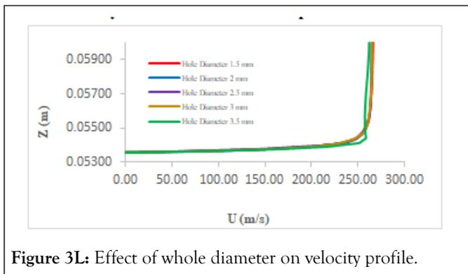
Figure 3L: Effect of whole diameter on velocity profile.
