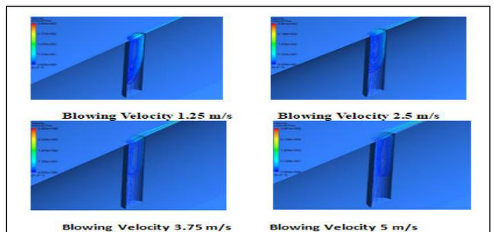
Figure 3G: The path line of the flow characteristics from the symmetrical plane micro-porous holes at variable blowing velocity.
