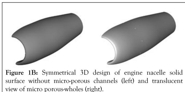
Figure 1B: Symmetrical 3D design of engine nacelle solid surface without micro-porous channels (left) and translucent view of micro porous-wholes (right).
