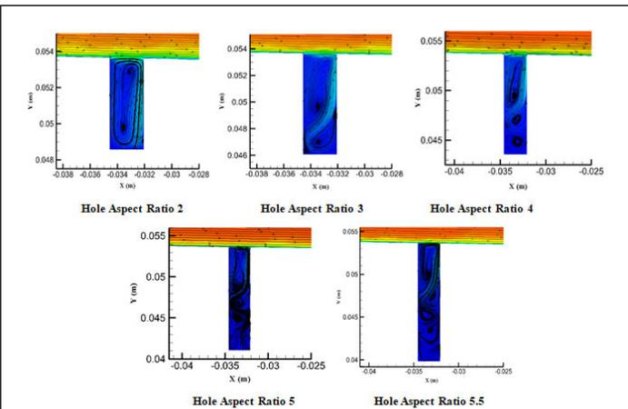
Figure 3H: Streamlines of the flow with variable whole aspect ratio and constant hole diameter with blowing velocity of 0 m/s around the micro-porous channel.
