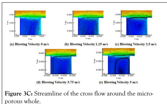
Figure 3C: Streamline of the cross flow around the micro-porous whole.
