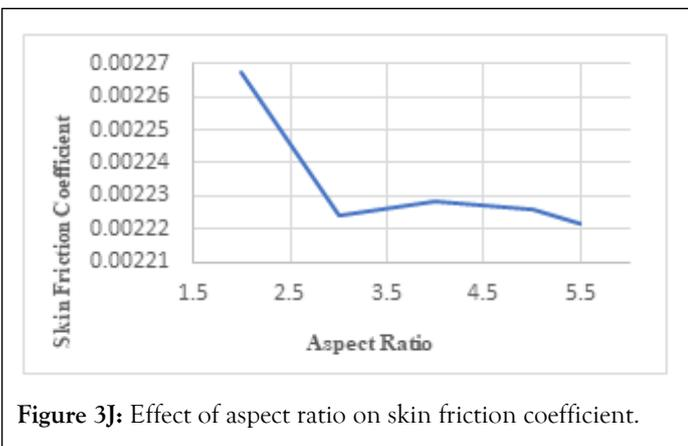
Figure 3J: Effect of aspect ratio on skin friction coefficient.
