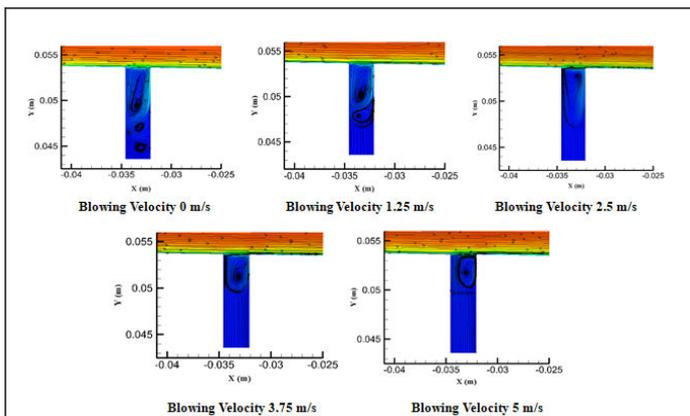
Figure 3D: Streamlines of the flow with variable blowing velocity around the micro-porous channel.
