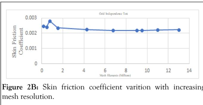
**Figure 2B:** Skin friction coefficient variation with increasing mesh resolution.
