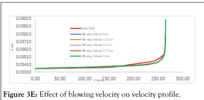
Figure 3E: Effect of blowing velocity on velocity profile.
