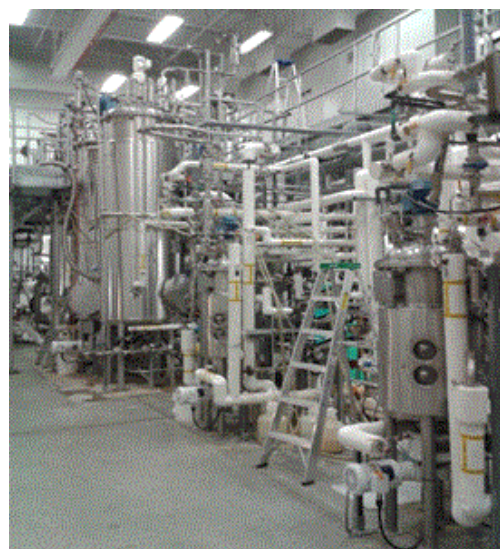
Figure 1: A portion of the pilot scale fermentation unit presently being used for Bacillus thuringiensis based bio-insecticide production at INRS-ETE, Canada.
