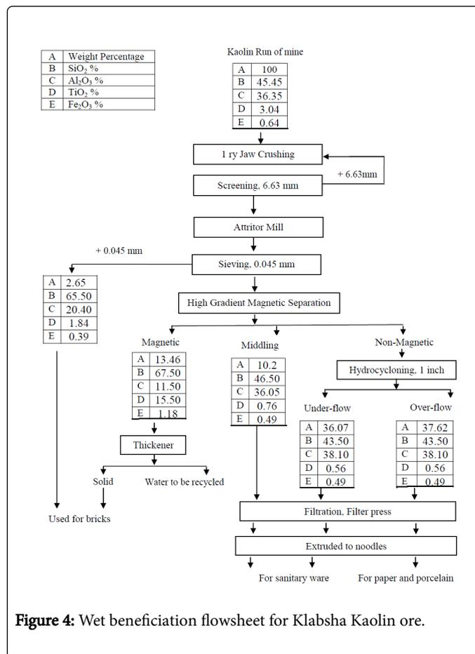
**Figure 4:** Wet beneficiation flowsheet for Klabsha Kaolin ore.
