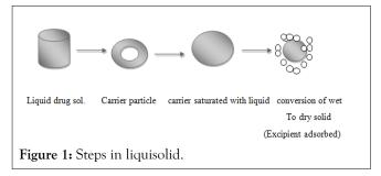
The wettability of the compacts by the dissolution media is one of the proposed mechanisms for explaining the enhanced dissolution rate from the liquisolid compacts. Non-volatile solvent present in the liquisolid system facilitates wetting of drug particles by decreasing interfacial tension between dissolution medium and tablet surface.
