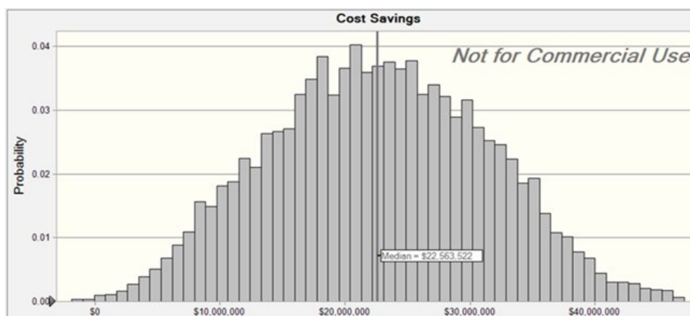
Figure 4: Cost savings/Monte Carlo simulation output with +/- 10% standard deviation for applied variables.
