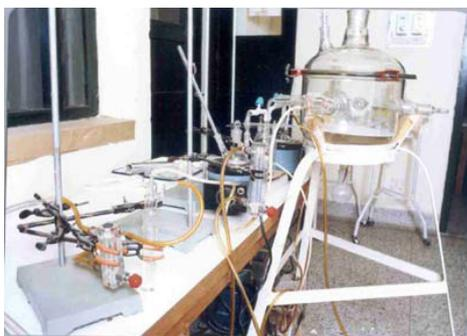
**Figure 1:** Inhalation assembly used for exposure of C-Compressed air only, F-furfural alone (95ppm), K-Kerosene alone (426-1054ppm), K+F-furfural and kerosene vapors (95ppm) and (426-1054ppm) respectively.
