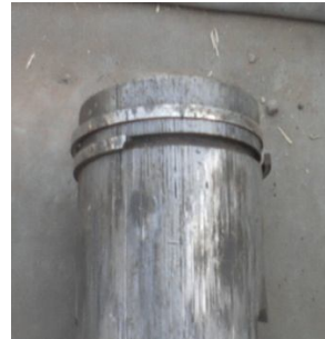
b) Inappropriate Piston or damaged piston Ring
