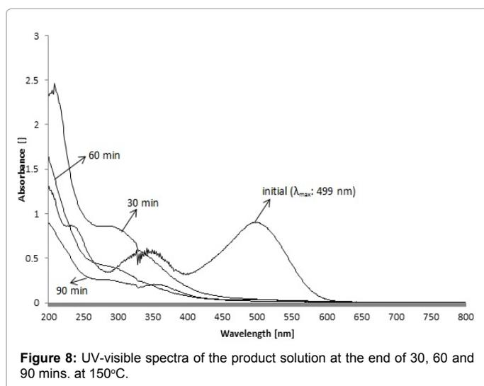
Figure 8: UV-visible spectra of the product solution at the end of 30, 60 and 90 mins. at 150°C.
