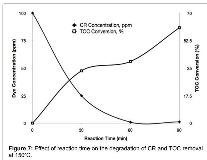
Figure 7: Effect of reaction time on the degradation of CR and TOC removal at 150°C.
