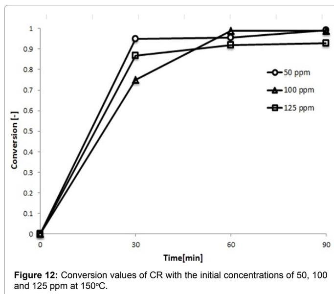
Figure 12: Conversion values of CR with the initial concentrations of 50, 100 and 125 ppm at 150°C.
