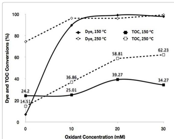
Figure 5: Effect of oxidant concentration on the conversions of CR and TOC at 150 and 250°C.
