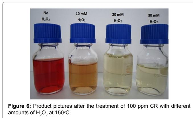
Figure 6: Product pictures after the treatment of 100 ppm CR with different amounts of H<sub>2</sub>O<sub>2</sub> at 150°C.
