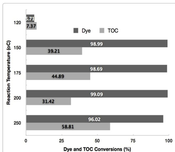
Figure 4: Effect of reaction temperature on the conversions of CR and TOC in the presence of 100 ppm dye and 50 mM  $H_2O_2$ .
