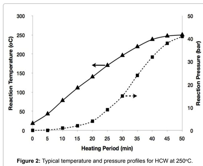
Figure 2: Typical temperature and pressure profiles for HCW at 250°C.
