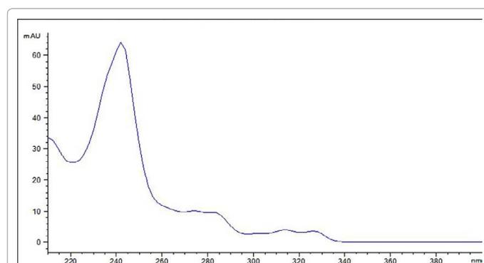
Figure 2: Absorption spectrum of halofuginone concentration of 1 mg / L in 0.25M acetate buffer
