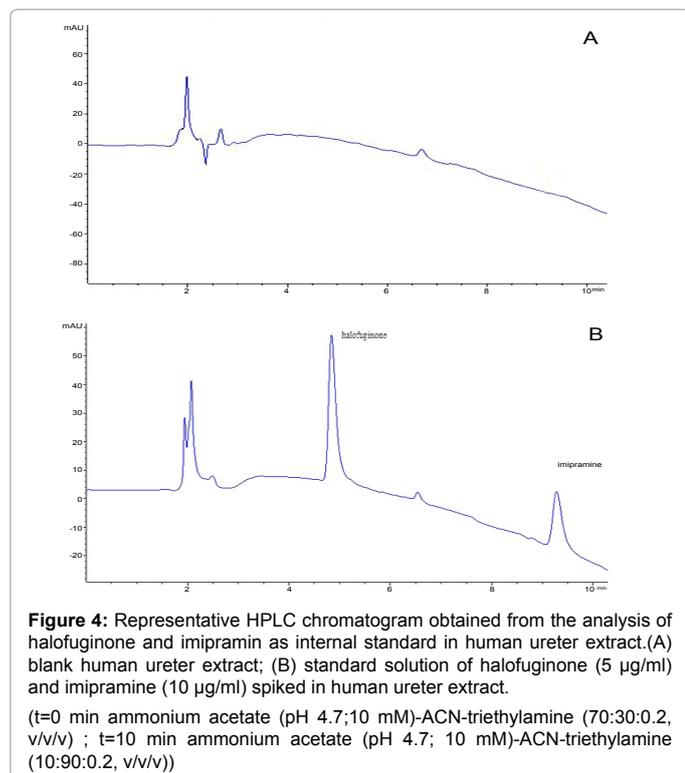
**Figure 4:** Representative HPLC chromatogram obtained from the analysis of halofuginone and imipramine as internal standard in human ureter extract. (A) blank human ureter extract; (B) standard solution of halofuginone (5 µg/ml) and imipramine (10 µg/ml) spiked in human ureter extract. (t=0 min ammonium acetate (pH 4.7;10 mM)-ACN-triethylamine (70:30:0.2, v/v/v) ; t=10 min ammonium acetate (pH 4.7; 10 mM)-ACN-triethylamine (10:90:0.2, v/v/v))
