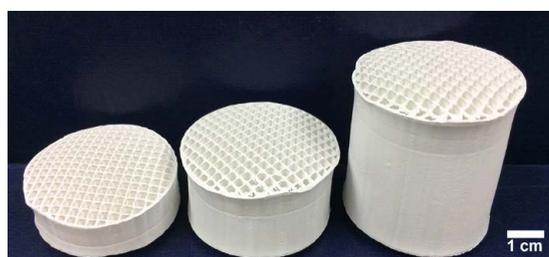
Figure 1: Honeycomb structures of S3 of different thicknesses after sintering at 800°C for 4 hours.
