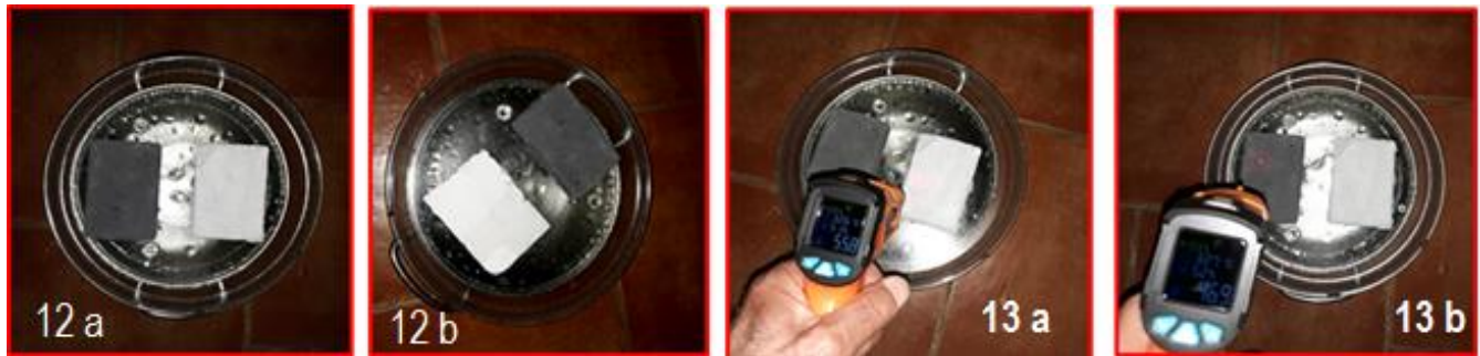
Figure 12 a: 'L1-B3' and 'L1-S3' on the hot pyrex lid; Figure 12 b: 'L1-B2/Lm' and 'L1-B2' on the hot pyrex lid Figure 13 a: T-reading on 'L1-B2' and 'L1-S2'; Figure 13 b: T-reading on 'L1-B3' and 'L1-S3'
