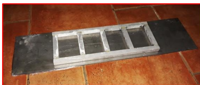
Figure 7: The 4-tile mould (in Aluminum) resting upon its steel base
