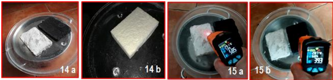
Figure 14 a: Tiles 'L3-C1-S10' and 'C1-B10' on hot pot lid; Figure 14 b: Tile of Stiferite on hot pot lid; Figure 15 a: T-reading on tile 'L3-C1-S10'; Figure 15 b: T-reading on tile 'L3-C1-S10'
