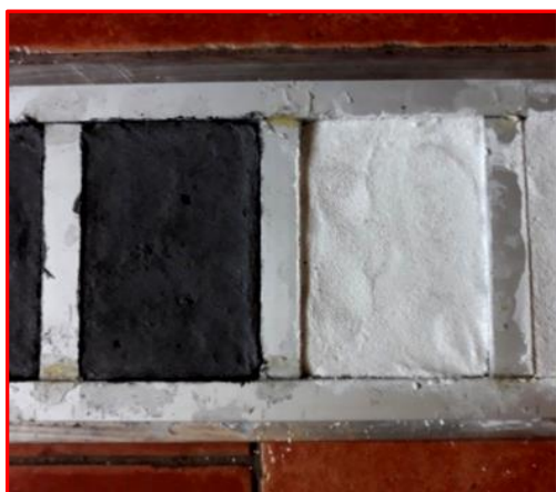
Figure 11: Tile 'L1-B2' at left vs tile 'L1-B2/Lm' at right: this latter appears full-white, due to 'lime-milk' coat
