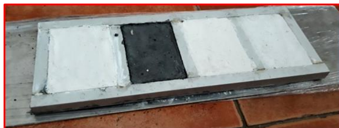
Figure 8: Different plasters as cast in the mould, undergoing curing.
