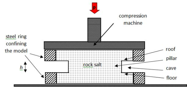
**Figure 5:** Pillar model, cross; derived from Lomineck and Bradshaw.
