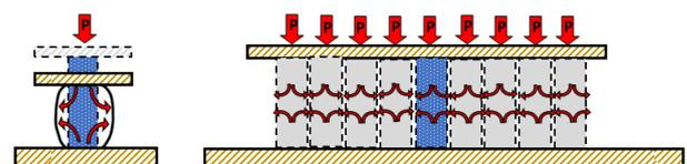
**Figure 3:** The mechanical behavior of a stand-alone small cylinder of rock under compressing stress  $P$ , compared with its mechanical behavior when embedded in a plate of rock under the same stress.
