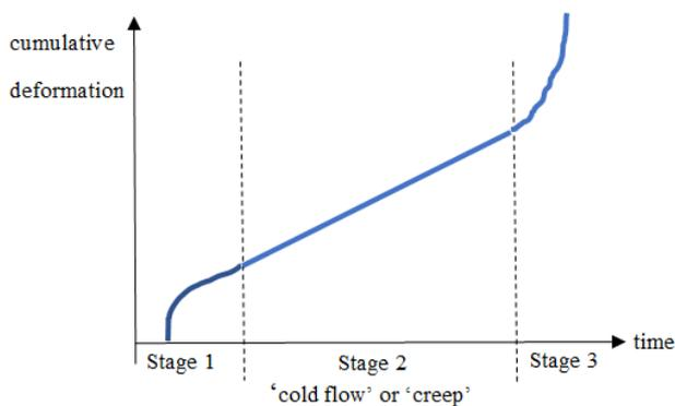
**Figure 2:** Deformation of a pillar of rock under a compressing stress.
