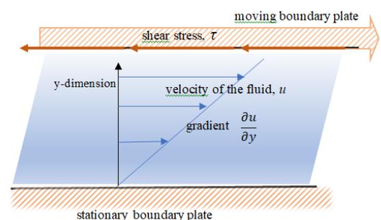
**Figure 4:** The change of the velocity of a fluid between a moving and a stationary boundary plate.
