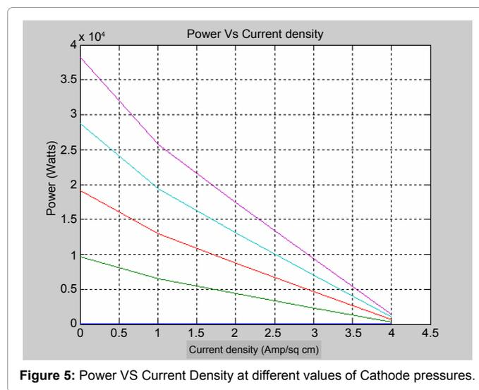
Figure 5: Power VS Current Density at different values of Cathode pressures.
