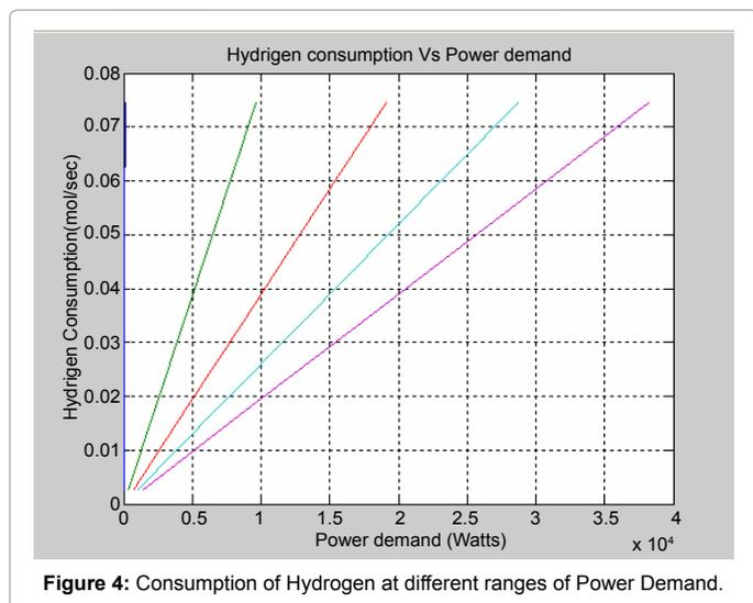
Figure 4: Consumption of Hydrogen at different ranges of Power Demand.
