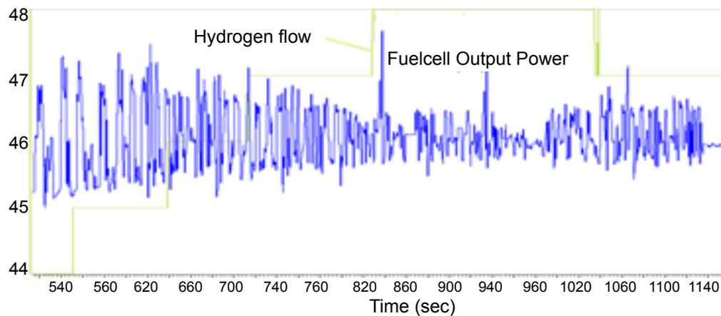
Figure 12: Hydrogen flow vs Fuel cell output Power.
