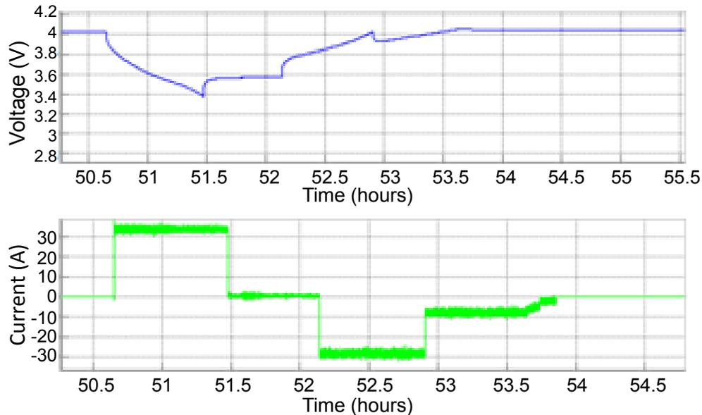
Figure 6: Constant current -Constant voltage Charging profile of Li-ion batteries.
