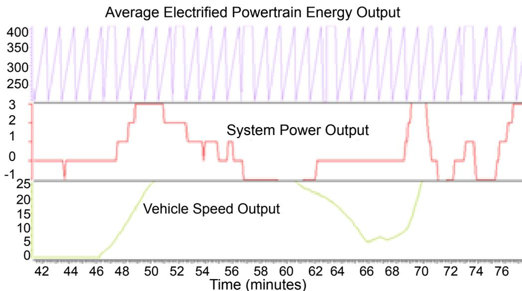
Figure 13: Average energy output and system power output in coherence with vehicle speed demand.
