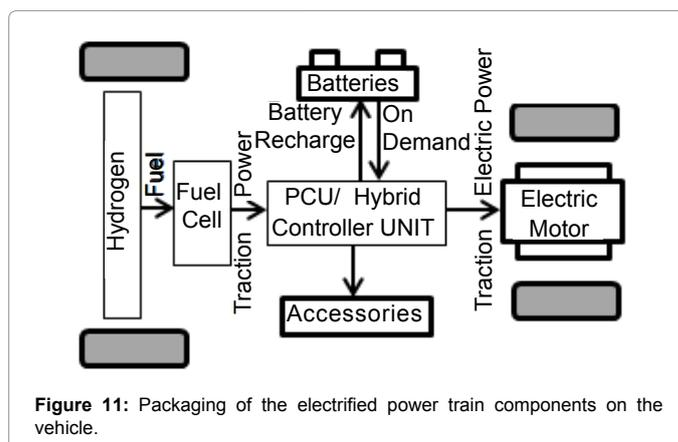
Hydrogen Cylinder=3,468.71 in<sup>3</sup>. So, the total space required=4,781.68 in<sup>3</sup>. The space on the trunk bed is equal to flat bed space area x height of flatbed = 70×48×12=40,320 in<sup>3</sup>. Luggage space left= 40,320–4,781.68=35538.32 in<sup>3</sup>. Thus, the calculations show that there will be sufficient space for the proposed powertrain without compromising
