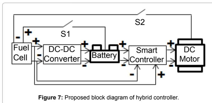
Figure 7: Proposed block diagram of hybrid controller.
