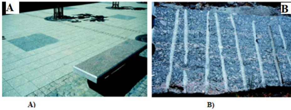
**Figure 2:** A) Polished surface of the variegated Babile granite (right) and flamed and honed tiles of the Porphyritic Anger Gutin granite (left) Sheraton hotel in Addis Ababa. B) Raw block surface of the Anger Gutin granite in the quarry (cut perpendicular to the foliation. Drill holes are approximately 25 mm wide.
