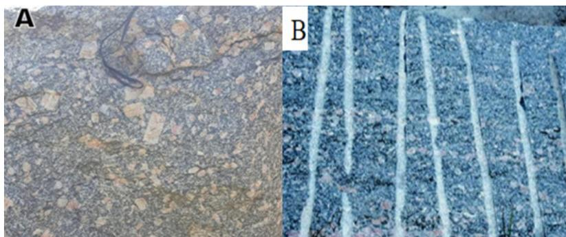
**Figure 4:** A) Granite rocks from Aba Musa area which is highly dominated by pink k-feldspar and B) Raw block fresh surface of the Anger Gute granite in the quarry (cut perpendicular to the foliation), drill holes are approximately 25 mm wide.
