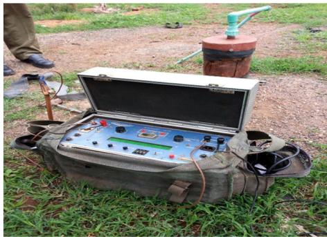
Figure 6: Geotron terrameter G41 model.
